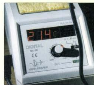
The temperature setting is digitally displayed on the SL30 solder station.
