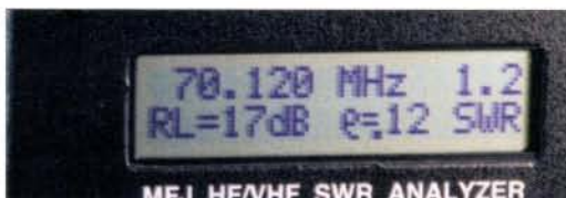
Fig. 7: The 98% transfer represents a return loss of 17dB between output and input.
