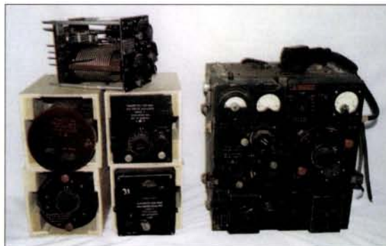
Fig 3: The T1083 transmitter with associated coils (see text).
