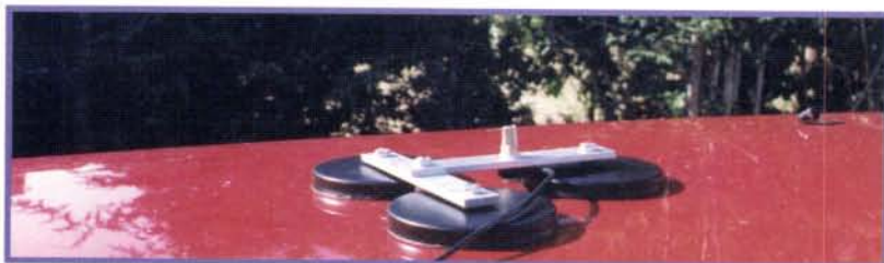
Fig. 1: Close up view of the MM-3401 triple magnetic mounting which proved more than capable of withstanding gale force winds (see text).
