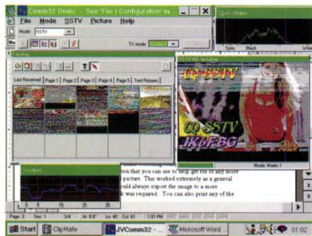
Fig. 2: The new JVcomm32 program receiving an SSTV image.
