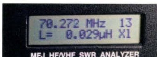
Fig. 5: ...or it might be an inductance of 29nH. Only further tests will establish what it actually is.
