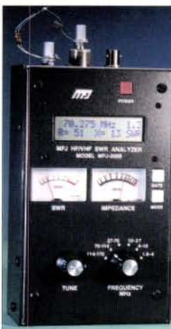
Fig. 2: The MFJ-259B in use testing a balun auto-transformer. (See text for more details).
