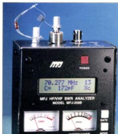
Fig. 4: The 13Ω reactive impedance of Fig. 3 , might be a 172pF capacitor...
