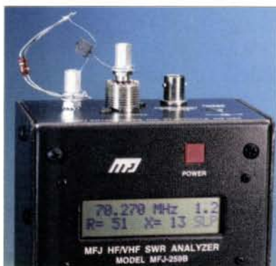
Fig. 3: The reflected resistance of the 190Ω load resistor combination should be 49Ω, but appears here as slightly high at 51Ω.
