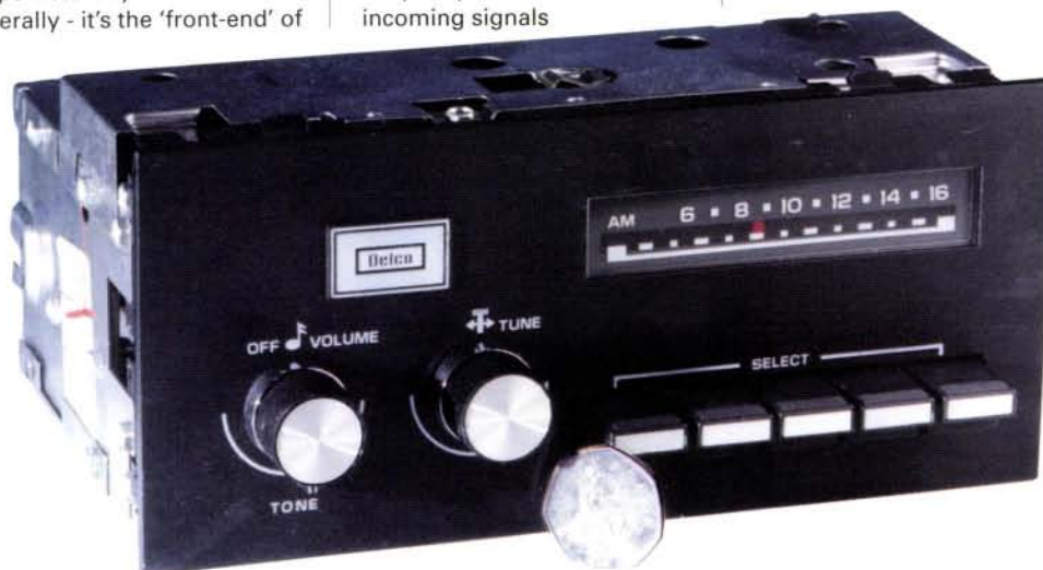
Fig. 1: The unusual 'Delco' (Made in Mexico for the American market) car radio which can be used as a 'tuneable intermediate frequency', photographed together with a 50p piece for size comparison. Looking almost like a miniature 'communications' receiver the radio is both sensitive and selective bearing in mind its original purpose.
