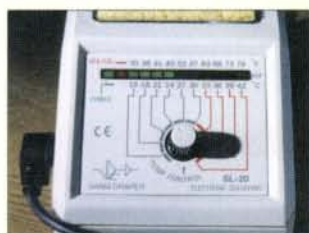
The temperature setting on the SL20 solder station, just below the bargraph row of l.e.d.s.
